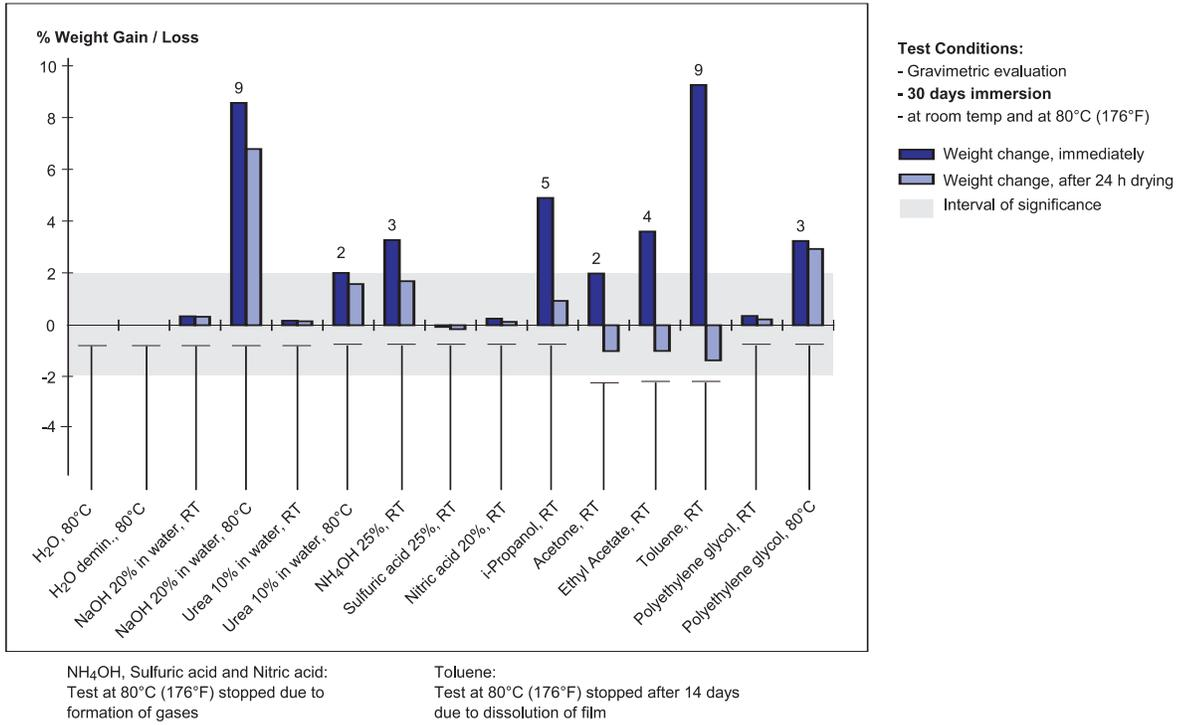
**FIGURE 2: Gravimetric Results After 90 Days of Immersion**
