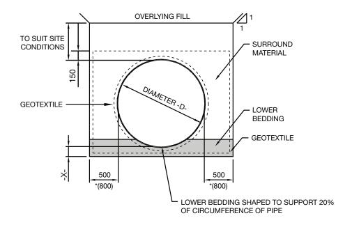
Minimum depth (X) of Lower Bedding material to be equal to Diameter (D) divided by 10. Therefore for a 1.8m pipe, X = 180mm. For a 2.4m pipe, X = 240mm etc.
